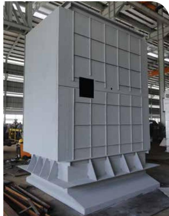
It is a solution that reduces a boiler's fuel consumption and improves its efficiency by using residual heat from its exhaust gas to heat its feed water.
